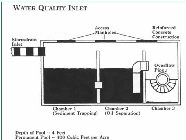
**An API separator is only partly effective at removing oily wastes, but is more effective at removing sediments than an ordinary catch basin**
