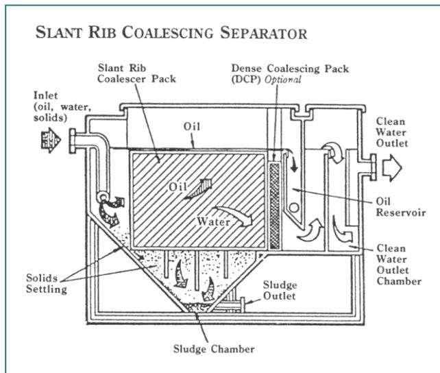
**A CPI separator can be very effective at removing oil but requires upstream sediment control and can be costly to maintain.**
