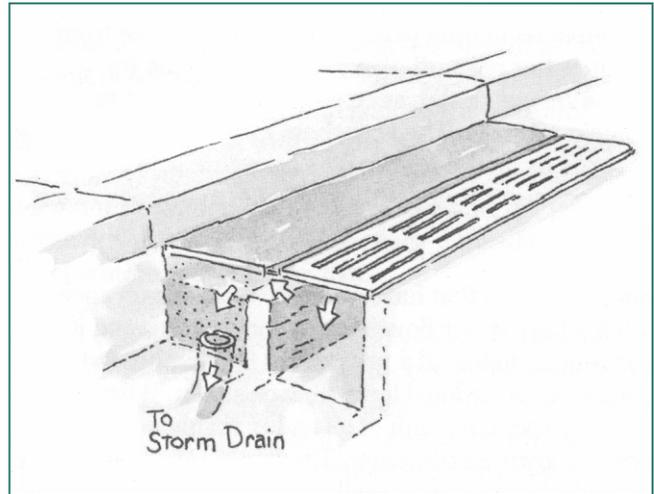
**A sand filter inlet can remove some pollutants before they enter the storm drain.**
