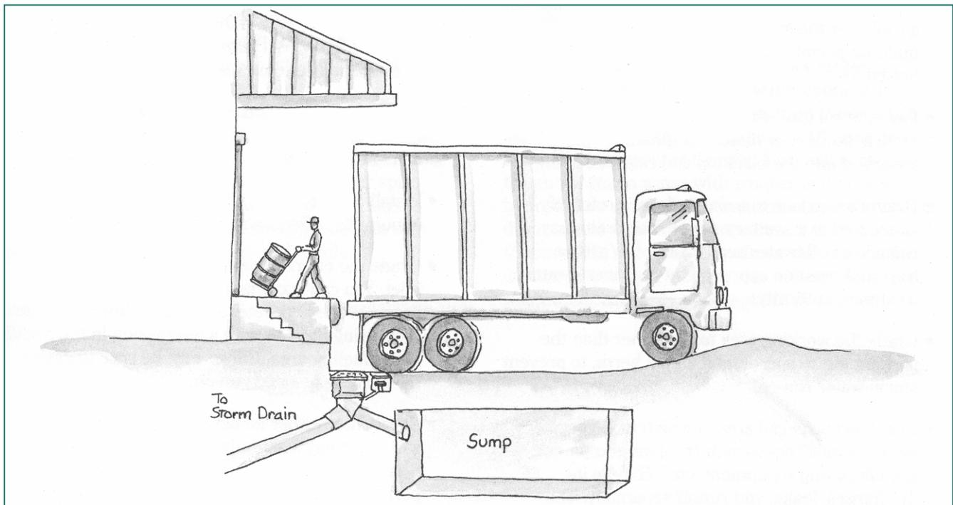
**A dead-end sump provides secure spill control, but any accumulated liquids need to be pumped out, tested, and properly disposed. Use berms or slopes to prevent run-on so storm water is not added to waste in the sump.**
